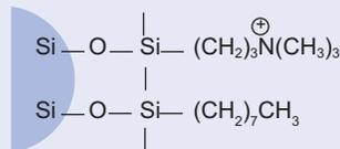
Chemical structure of SAX (Trimethylaminopropyl) silane and C8 (Octyl) silane, covalently bonded to the surface of a silica particle.
