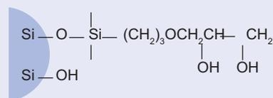
Chemical structure of Diol (2,3-Dihydroxypropoxypropyl) silane, covalently bonded to the surface of a silica particle.
