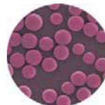
Silica packing, 5 \mu\text{m}
